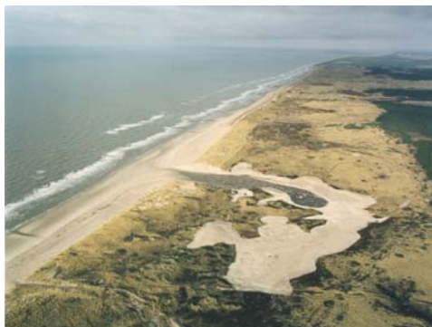
Figure 3. An artificial breakthrough of the front dunes to stimulate ecological diversity (sea water can enter from time to time) and nature values in the dunes. First example of dynamic management. De Kerf 1997.
