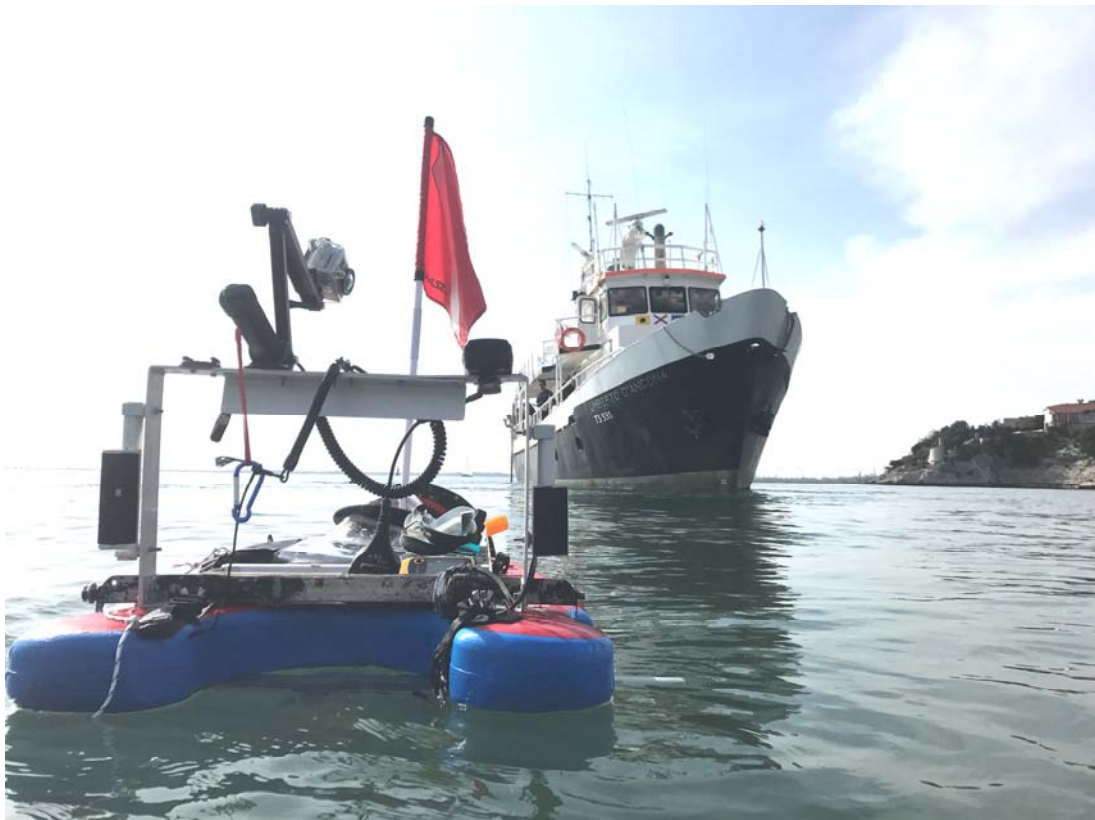
Figure 1. The 1.2 m-long raft, called “Barchino”, used for the snorkel surveys. Here the raft during a surveying test along the coastal sector between Sistiana and Duino, Gulf of Trieste (Italy).
