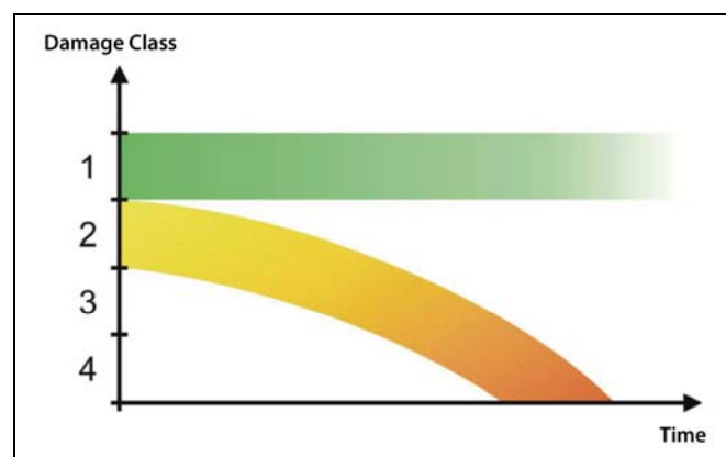
Figure 1. Damage classes versus time (according to BAW, 2011).
