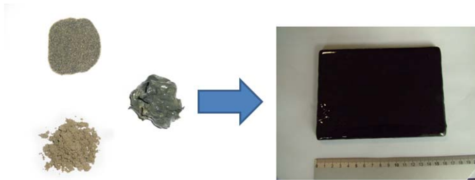
Fig. 2. Picture of black glass due to the dark sand and the presence of Fe 2 O 3 and MgO.
