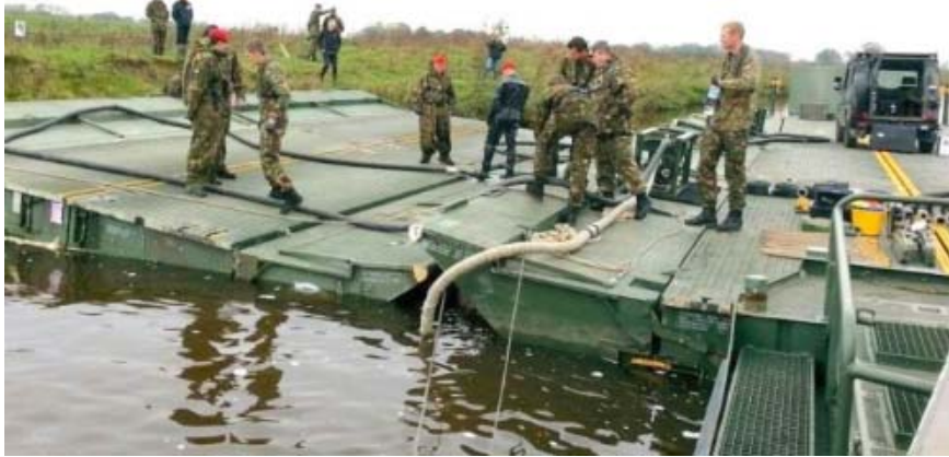
Figure 10. Multifunctional military pontoon BreachDefender.
