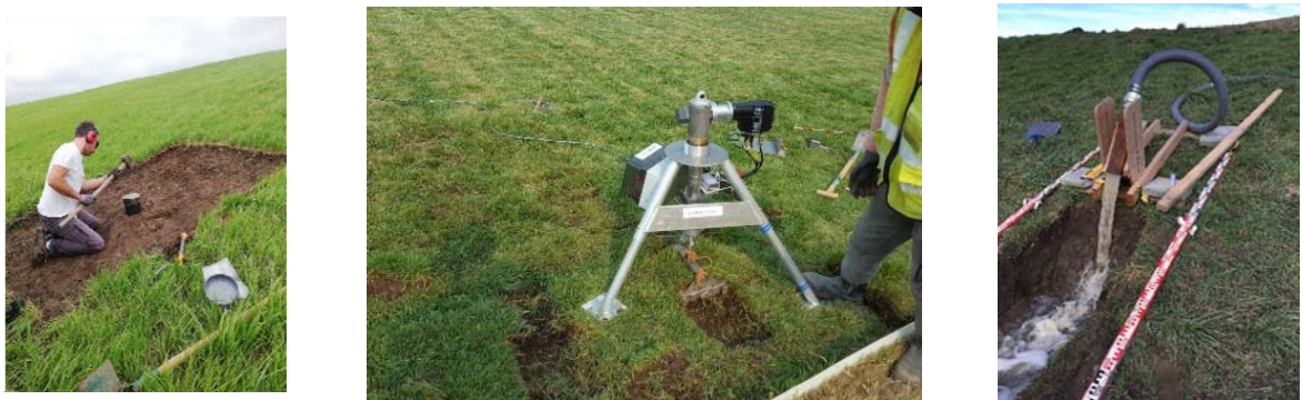
Figure 5. Sampling for JET-experiments (left), Grass Sod Pull test (middle), Fire Hose test (right).
