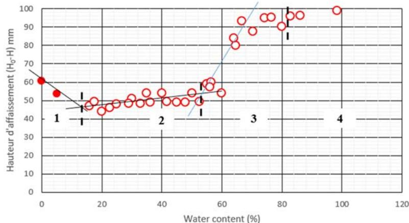
Figure 3. Slump (A) vs water content ( $w$ ) for Cherbourg harbor sediments.
