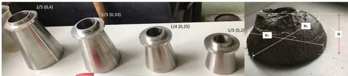
Figure 2. Abrams reduced scaled cones and measurement slump parameters.
