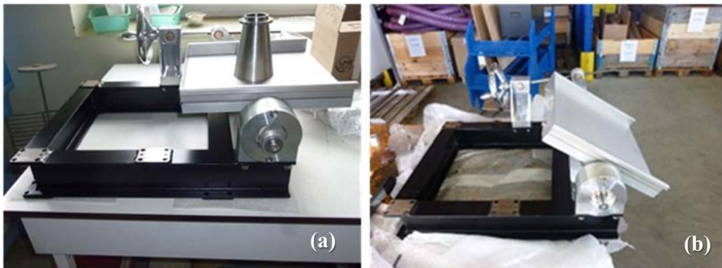
Figure 1. The shovel ability meter with the cone (left) and in sliding position (right).
