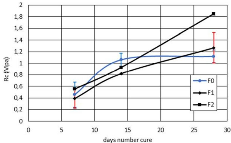
Figure 6. Compressive strengths of tested formulations.
