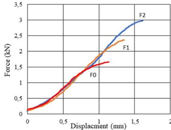
Figure 5. Stiffness of specimens treated with the three formulations.
