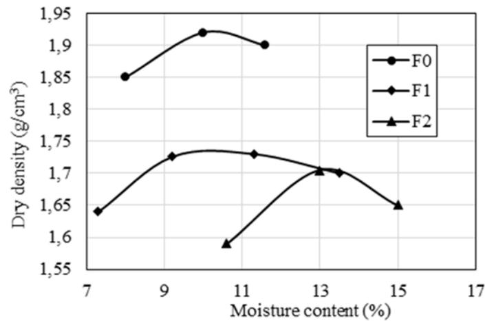
Figure 4. Compaction parameters of treated sediments.
