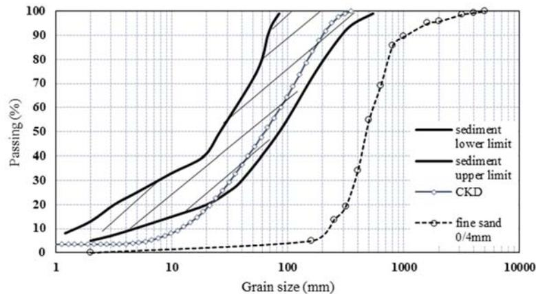
Figure 3. Grain size distributions of sediments, CKD and sand.
