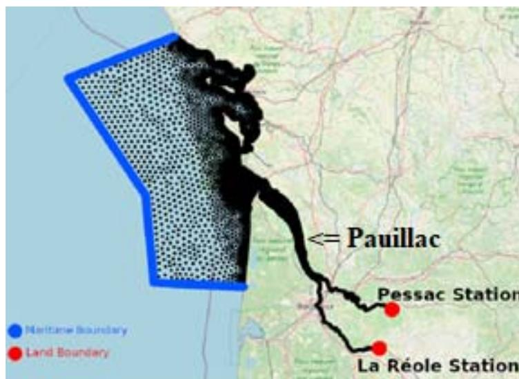
*Figure 1. Telemac3D model mesh developed by Cerema with the boundary conditions labelled.*
