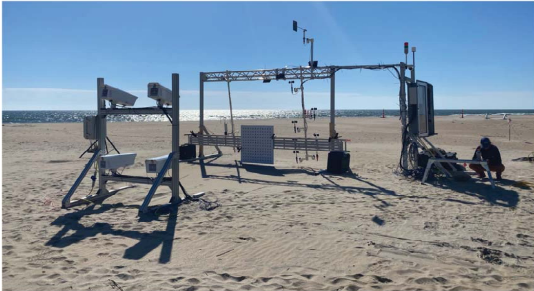
Figure 14. Picture of the F-PTV system on the beach at Wallops Island. Weatherproof cabinet shown on right attached to the instrumentation gantry.
