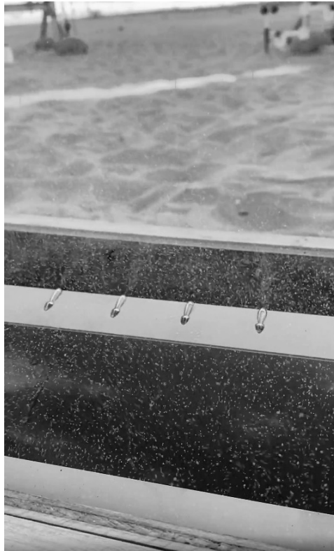
Figure 12. Helium Filled Soap Bubbles being generated from Linear Nozzle Array.
