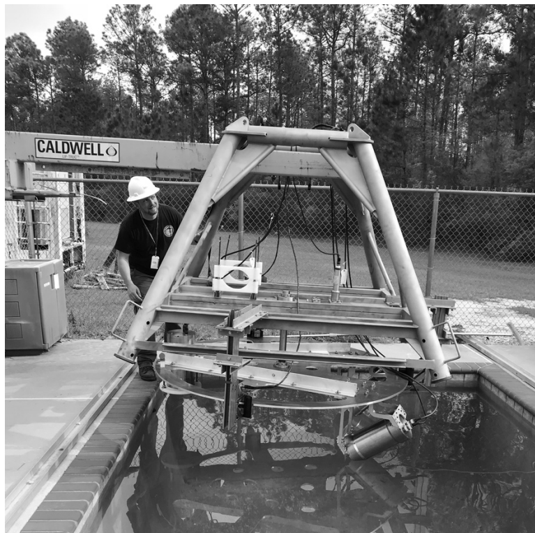
Figure 6. Immersion test of system at Stennis Space Center.
