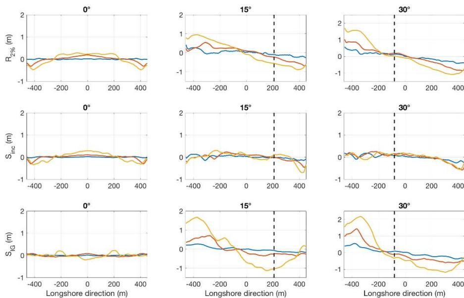
Figure 2. Longshore anomalies (difference between the local value and the mean longshore value) of  $R_{2\%}$ , the significant swash height IG  $S_{ig}$  and incident  $S_{inc}$ . Curve color: blue: moderate, red: high, yellow: storm, black dashed line: geometric shadow.
