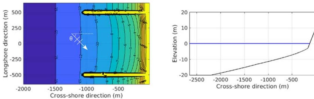
*Figure 1. Contour lines of the bathymetry (area of interest) exposed to waves with an angle of incidence  $\theta$  (left) and cross-shore transect in the middle of the embayed beach (right). The incident swell direction varies between  $0^\circ$  and  $30^\circ$ .*
