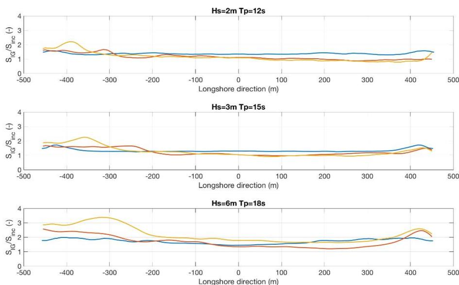
*Figure 3. Longshore evolution of the ratio  $S_{ig}$  over  $S_{inc}$  for the different conditions. Curve color: blue:  $0^\circ$ , red:  $15^\circ$ , yellow:  $30^\circ$ .*
