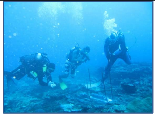
Figure 5. Installation of the SBE26+gauge on the sea bottom.
