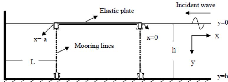
Figure 1. Schematic diagram for floating elastic plate connected with mooring lines.
